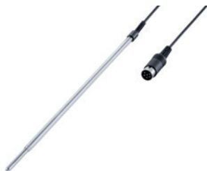
PT 1000.70 temperature probe, glass-sheathed for use in aggressive media such as acids and alkalis. Material: Borosilicate glass: 3.3. Ident. No.: 0003736000
